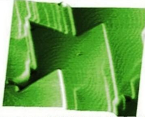
CdF 2 films grown on a CaF 2 (111) substrate. Scan is taken in contact mode using a CSC21 probe (now upgraded to HQ:XSC11). Scan size 2 x 2 μm, height 2 nm..
